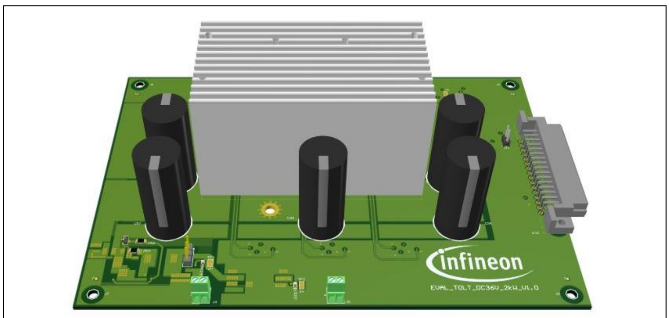
Figure 1 Isometric image of evaluation power board (EVAL_TOLT_DC36V_2KW V 1.0)
